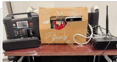
[ wheelchair-mounted sensing rig — 77 GHz radar, RGB-D camera, Jetson Orin Nano ]
